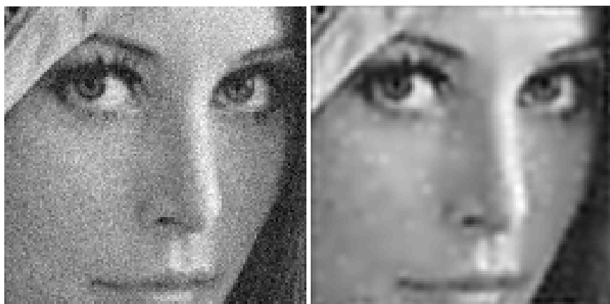
Fig. 2. LEFT: An 128 \times 128 image with added gaussian noise. RIGHT: Estimate of the DFT-RVM algorithm using gaussian kernels with variance 2, 4 and 8.
